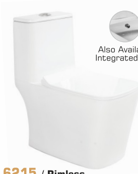
6215 / Rimless 670x360x740mm 26"x14"x29" Roughing in-S-Trap 200 / 300mm P-Trap 180mm Softclose Seat Cover, Dual Flush Kit
