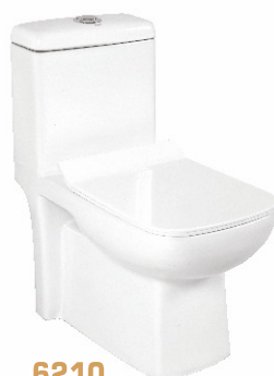
6210 670x350x750mm 26"x14"x30" Roughing in-S-Trap 300mm P-Trap 180mm Softclose Seat Cover, Dual Flush Kit
