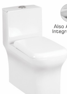
6160 640x360x720mm 25"x14"x28" Roughing in-S-Trap 230 / 300mm P-Trap 180mm Softclose Seat Cover, Dual Flush Kit
