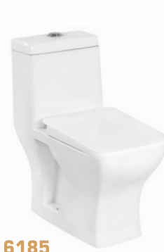
6185 660x360x750mm 26"x14"x30" Roughing in-S-Trap 200mm P-Trap 180mm Softclose Seat Cover, Dual Flush Kit
